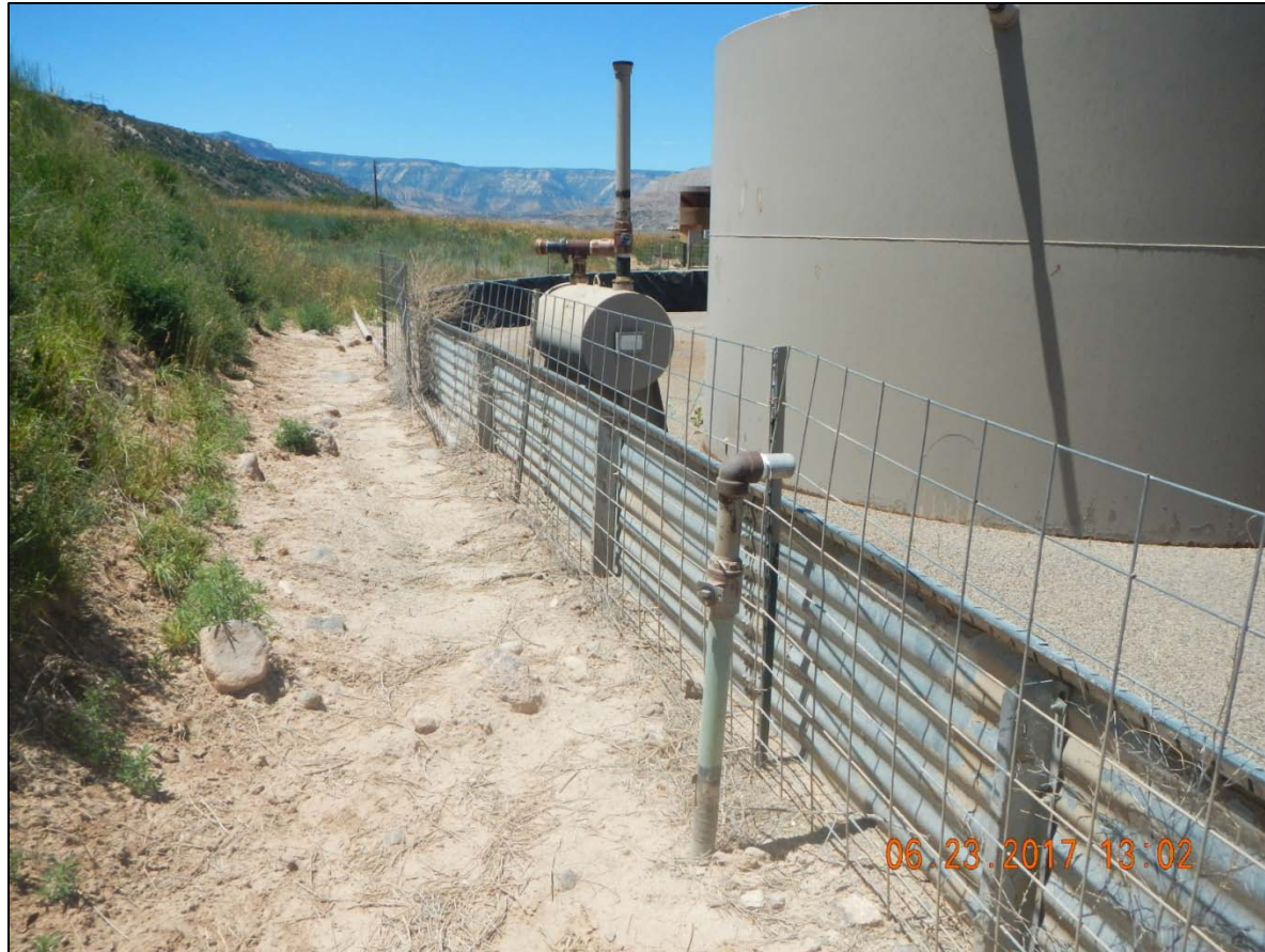
Unused 2" riser behind tank battery
