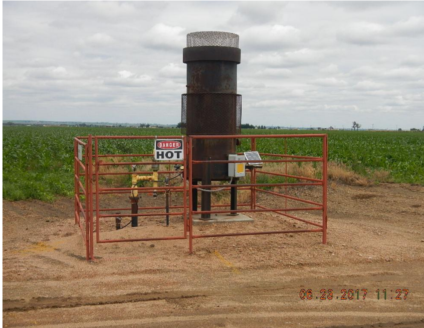
Photo 3 Emission Control Burner from south
