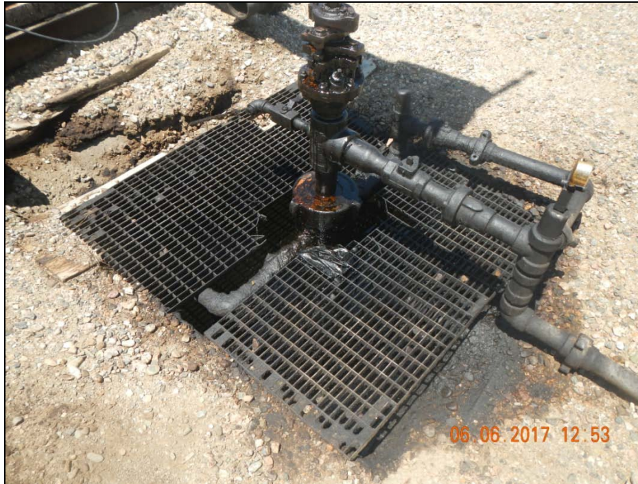
Photo 1. Cellar fully of oily fluid without 2 feet of freeboard.
