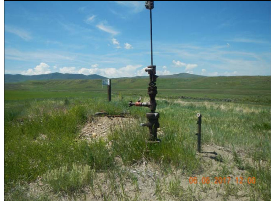
Photo 2. 1 – 2" steel riser at wellhead not marked for abandonment.
