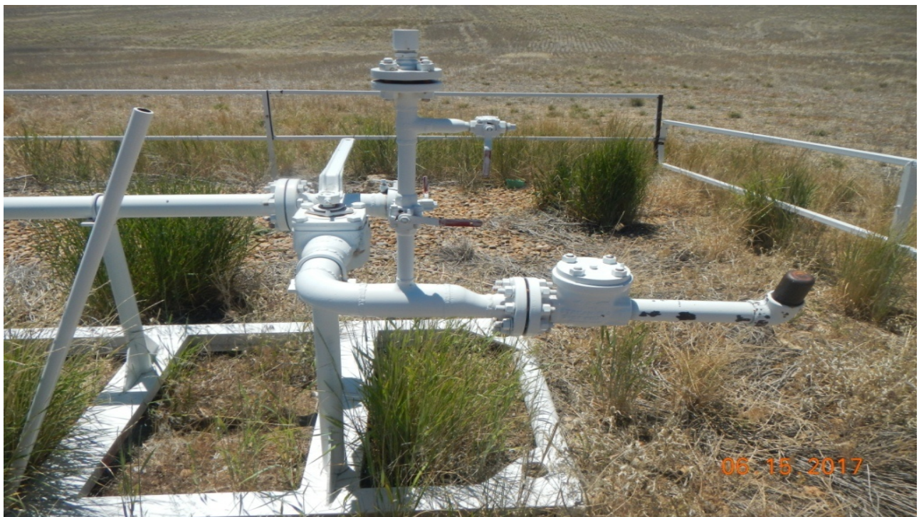
photo 2: There has been no lock out/tag out applied to the valve levers.
