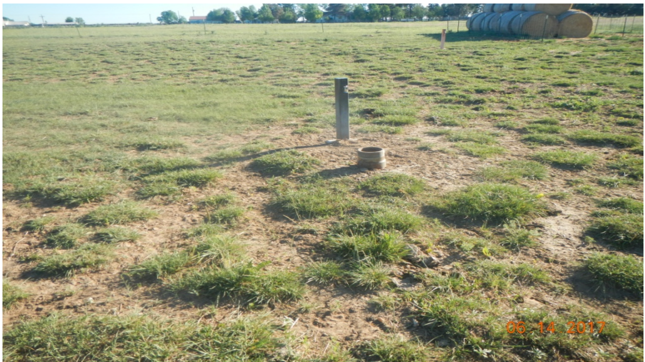
photo 4: There are numerous square pipe in the ground at the location which appears to be for groundwater monitoring.
