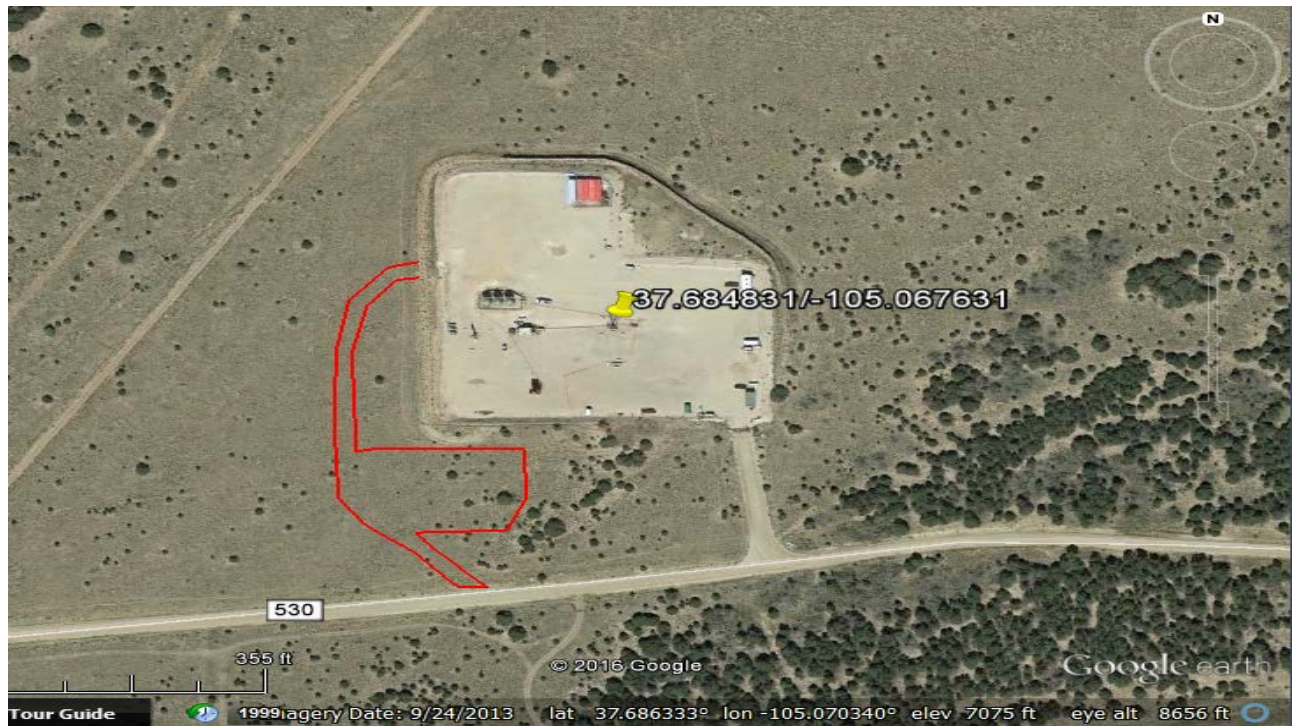
photo 1: Aerial photo 2013 of the Freeman 3-24 location. The red outline shows approximate area of new disturbance. There were no stormwater controls in place.
