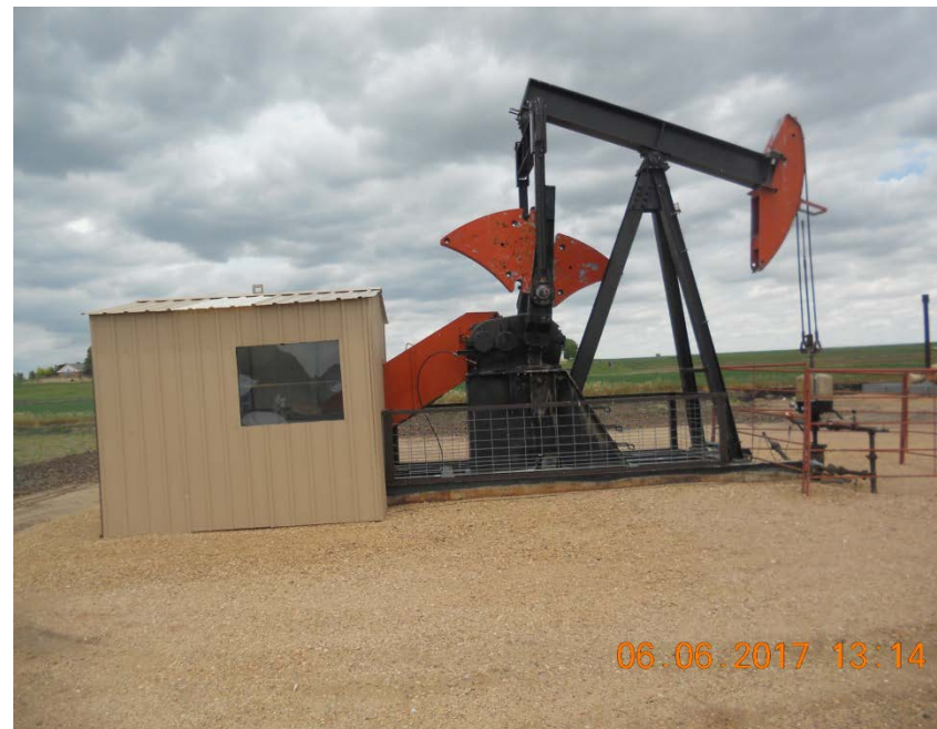
Wellhead and pumpjack looking north. Note no well sign visible
