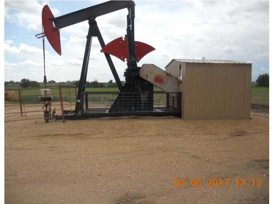
Wellhead and pumpjack looking south. Note no well sign visible
