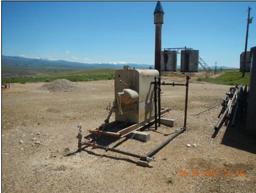
Photo 7. Horizontal heated separator with risers.
