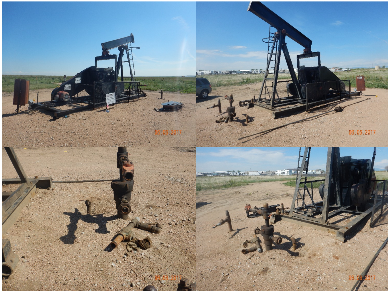
Photos 2, 3, 4, & 5 - Pumping unit and wellhead are currently disassembled, rendering well incapable of production. Note absence of bullplugs on wellhead and flowline risers. Flowline risers are out of compliance with 2017 Flowline NTO.
