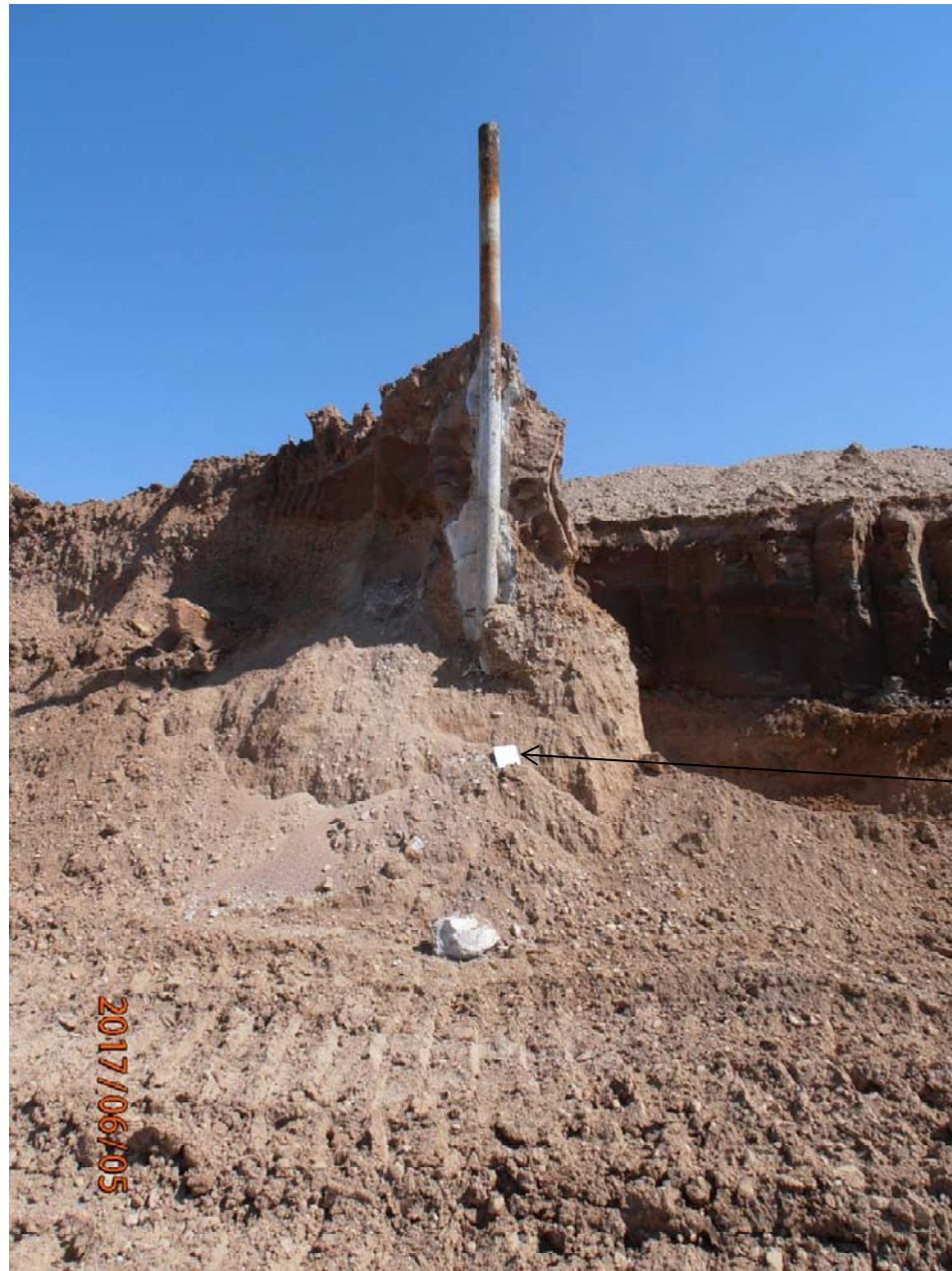
Casing of plugged and abandoned Loloff-Sand 1 in active gravel pit. 8 ½ x 11 notebook for scale.
