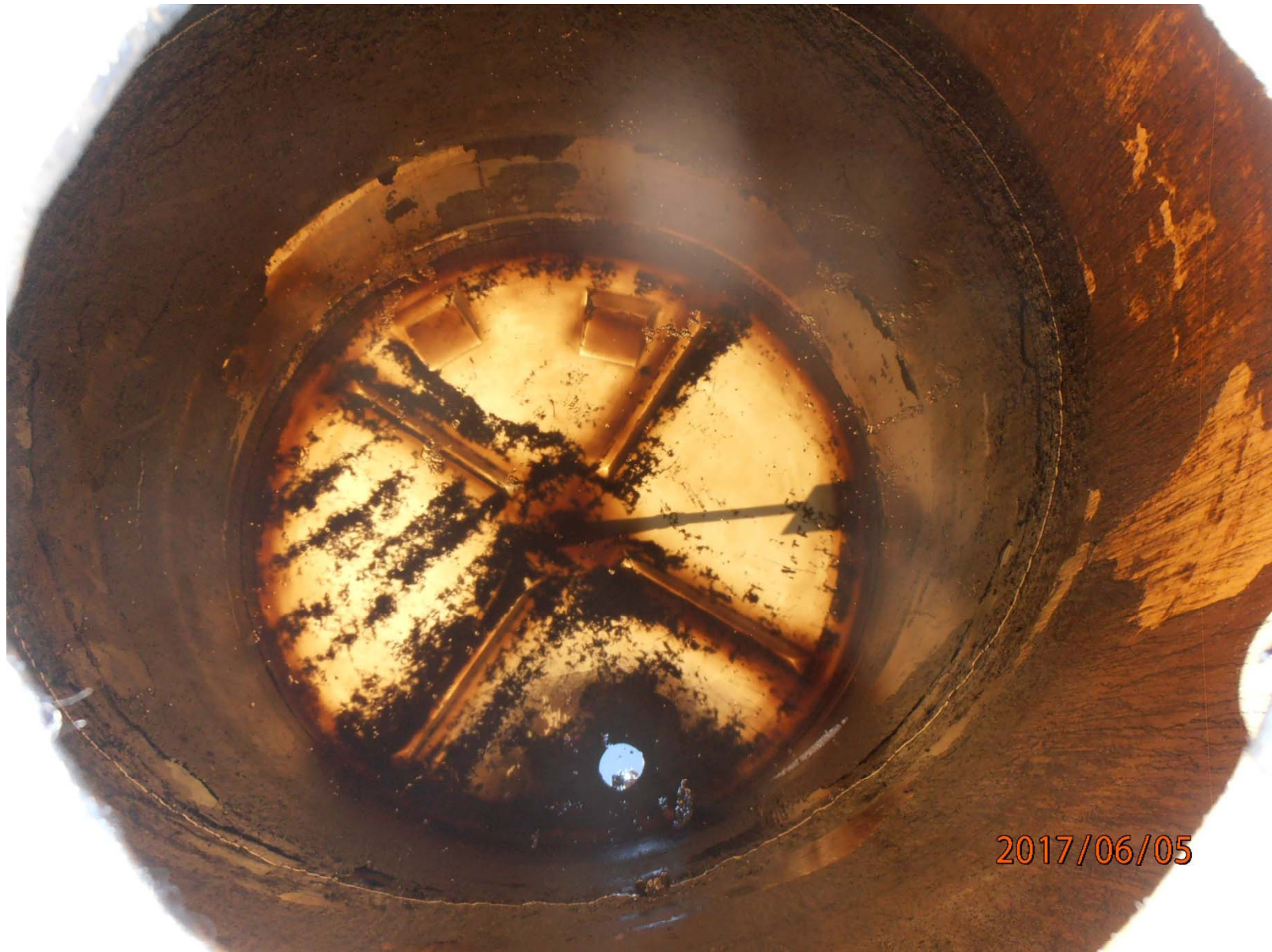
Water present in former produced water vessel.
