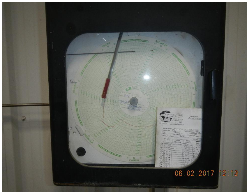
Photo 1 Pressure chart inside pump house Inj Tubing 900 psi
