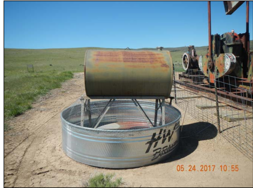
Photo 4. Unlabeled methanol tank.
