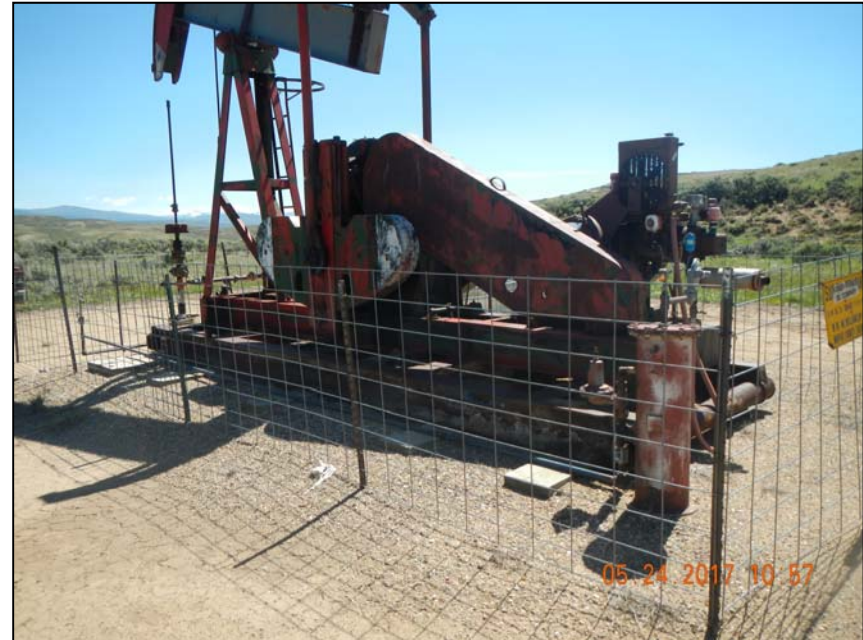
Photo 6. 1 – 1" steel line to separator and 1 1" poly line to motor.
