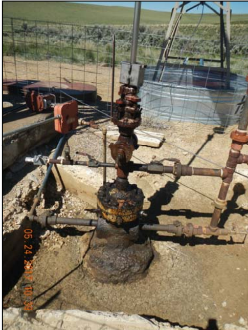
Photo 3. Stained soil at wellhead.
