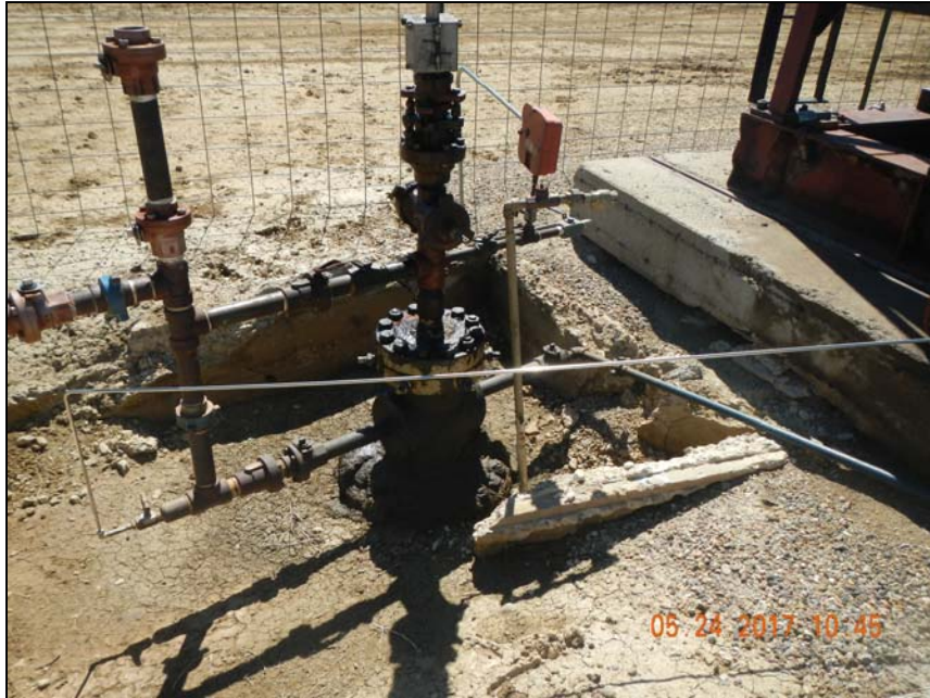
Photo 5. 1 -1" steel riser not in use, alternate angle.
