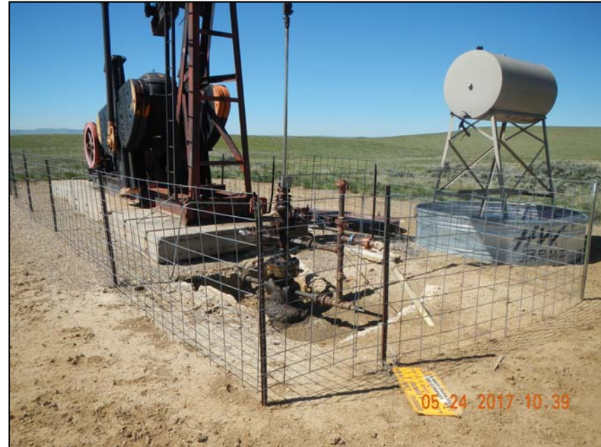
Photo 2. Overview of wellhead assembly with fallen wellhead sign and unlabeled methanol container visible.
