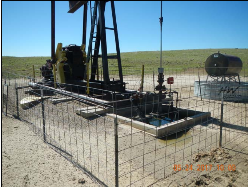
Photo 3. Lines going to separator and motor. Unlabeled methanol tank.
