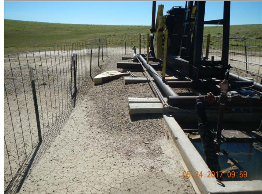
Photo 2. 1" steel flowline from wellhead to separator.
