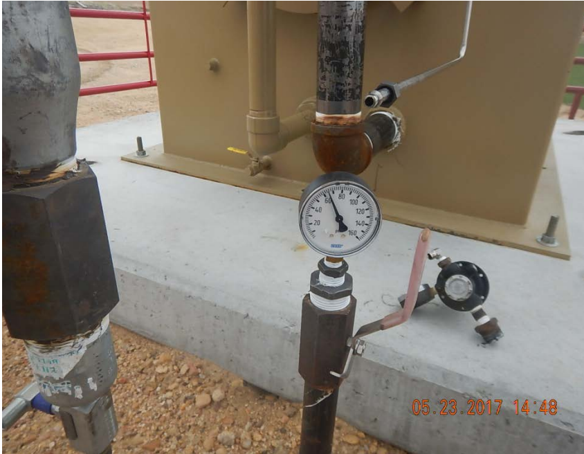
Photo 1: Pressure test on ECD supply line
