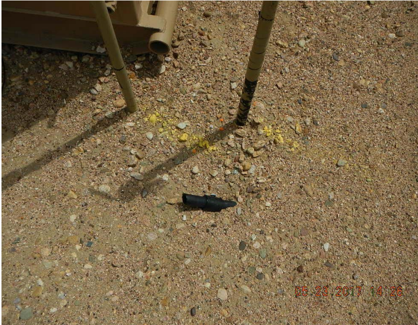
Cut 1" poly process line N40.32746 W-104.83073
