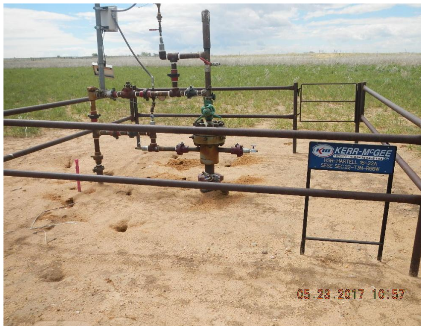
HSR – Hartell 16-22A Wellhead with capped and painted riser. From north
