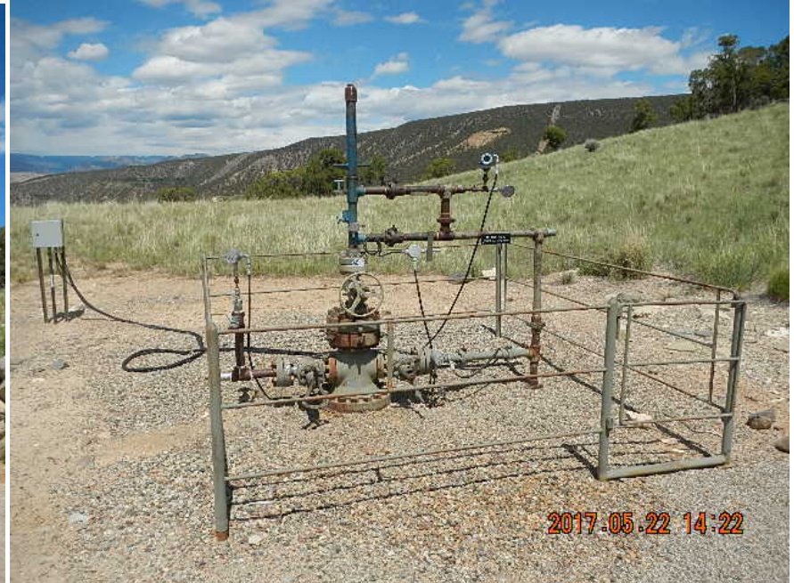
1-2" steel line from wellhead to separator.
