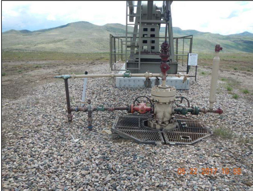
Photo 2. 2 -2" steel risers at wellhead.
