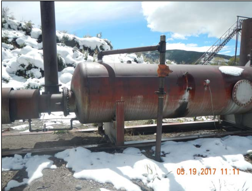
Photo 7. 2" steel riser at separator.
