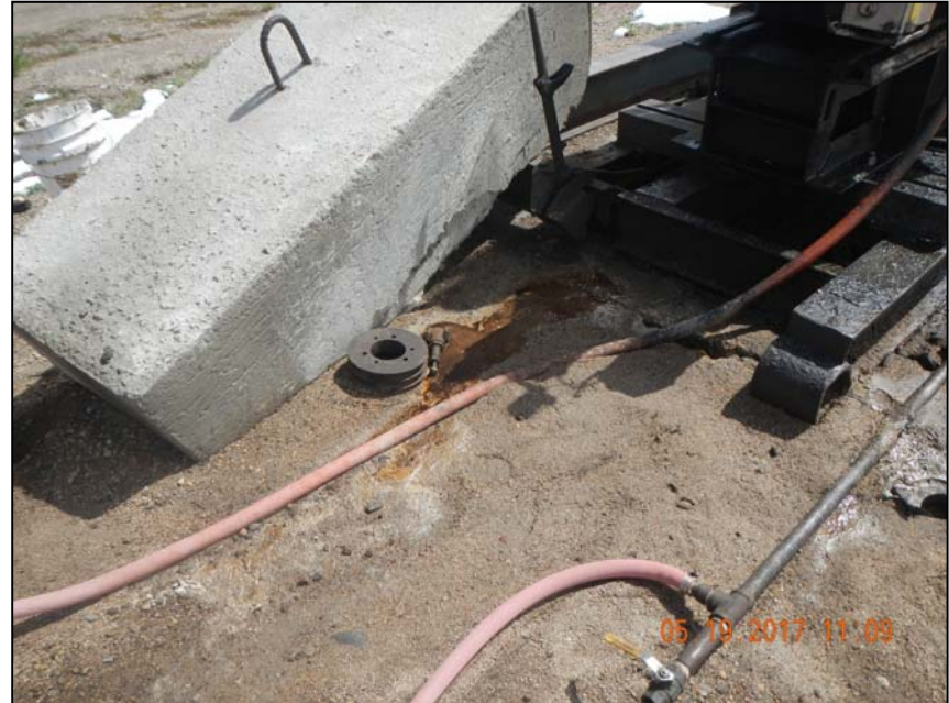
Photo 6. Oil leaking from rear of pump jack motor.
