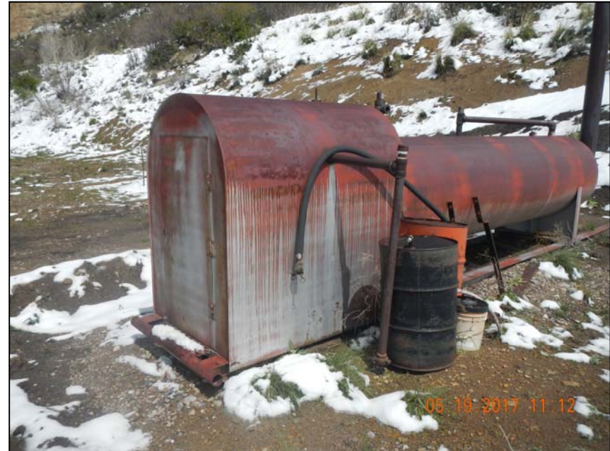
Photo 8. 3" steel riser at separator.
