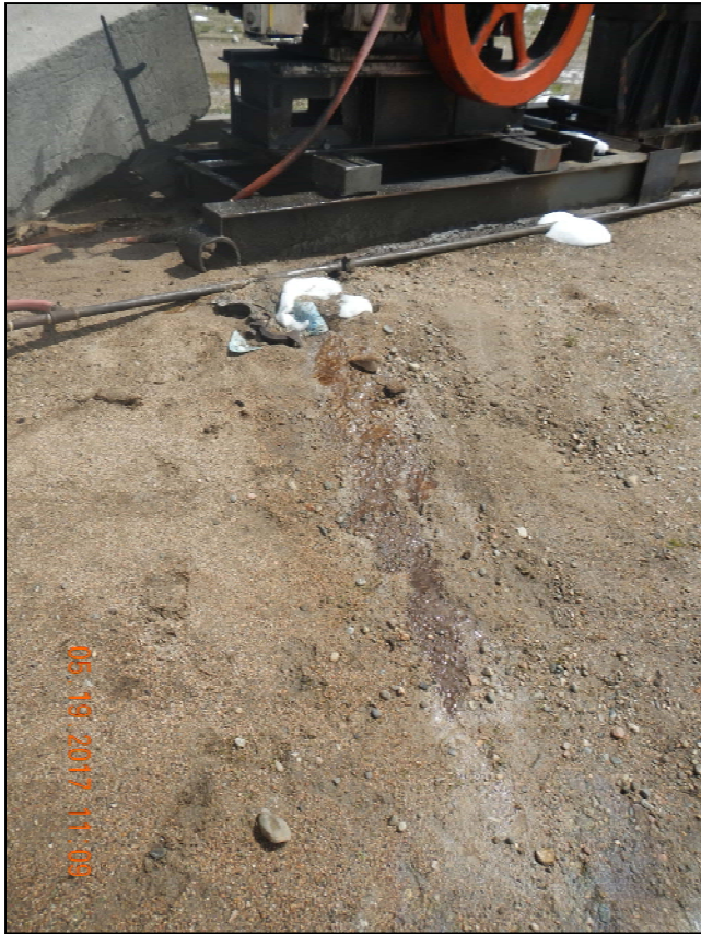
Photo 5. Lube oil leaking from side of pump jack motor.
