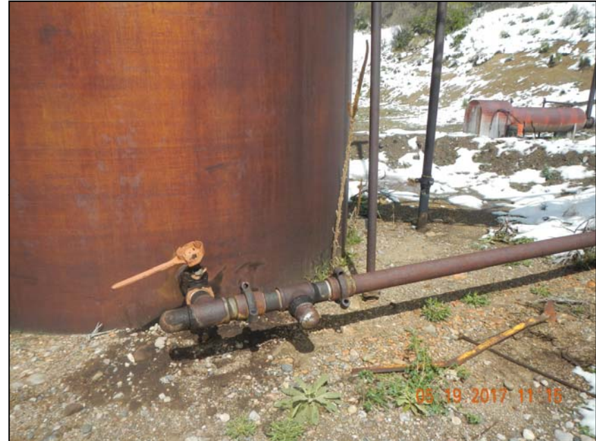
Photo 10. Stained soil at tank base. 2", 3" 4" steel flowlines.
