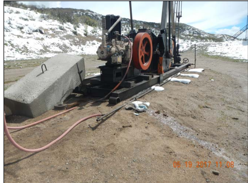
Photo 2. 1" steel flowline from wellhead to separator.
