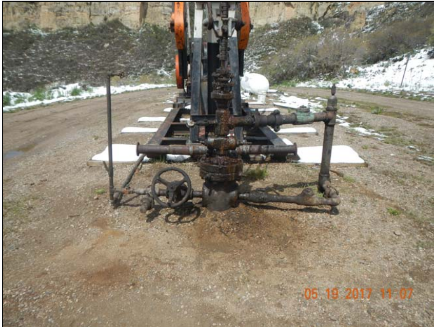
Photo 1. Wellhead with 2 steel risers. 1" on left 2" on right.
