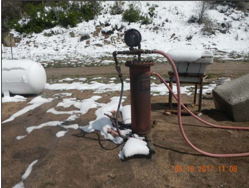
Photo 3. Separator for casing gas with 2 - 1" poly lines. One going to propane tank one going to pump jack motor.
