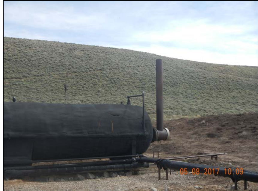
Photo 3. No wildlife protection apparent on exhaust.
