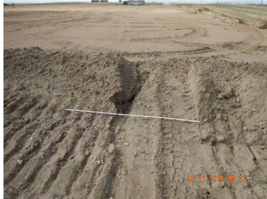
Photo 18: Photo taken from the northwest end of the location. Photo shows stormwater erosion has degraded the berm and slope of the location. Berms do not appear to be sufficiently consolidated on this area of the location. Vehicle traffic appears to have rendered the berm inadequate and allowed for stormwater degradation. 6 foot measuring stick for reference.
