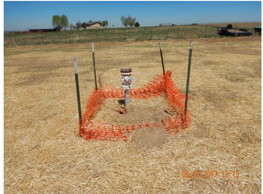
Photo 2. Close-up photo of the pipeline riser that remains at location.
