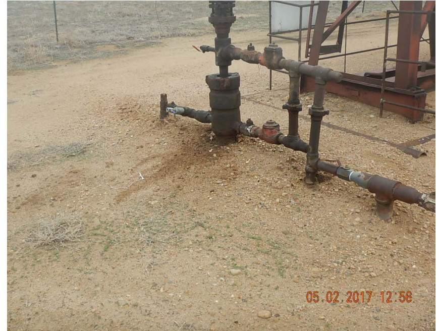
Photo 3: Stained soil at wellhead, bradenhead not plumbed to surface.
