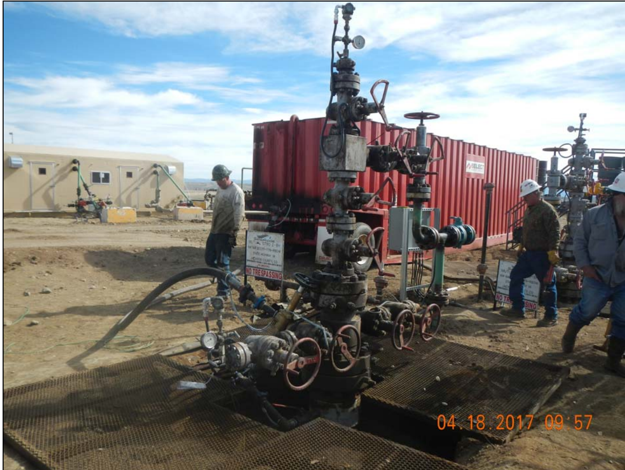
Photo 1. View of wellhead assembly prior to beginning of test.
