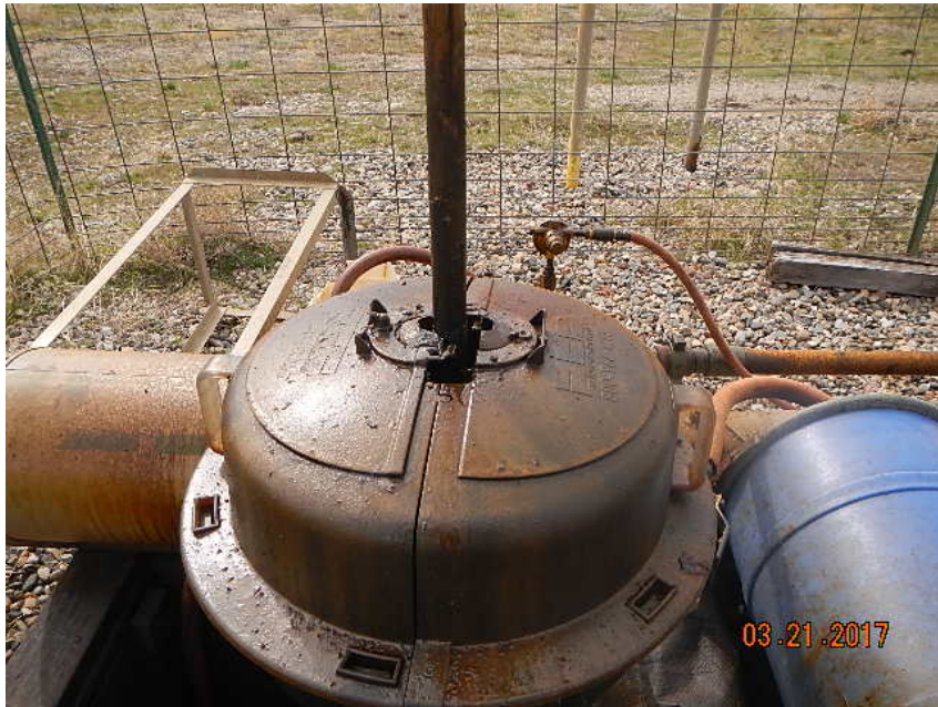
Photo 1. Stuffing box leaking condensate.
