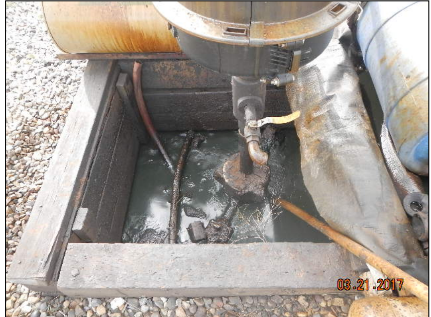
Photo 2. Containment under stuffing box.
