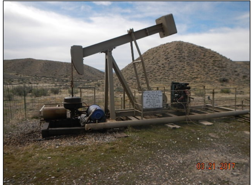
Photo 4. Pump Jack operating at time of inspection.
