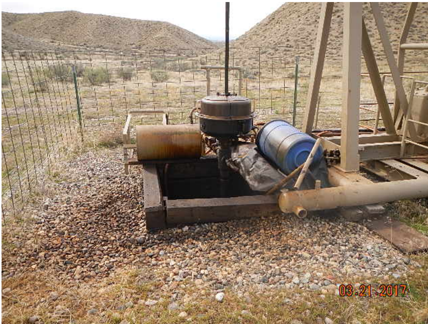
Photo 3. Staining around containment.
