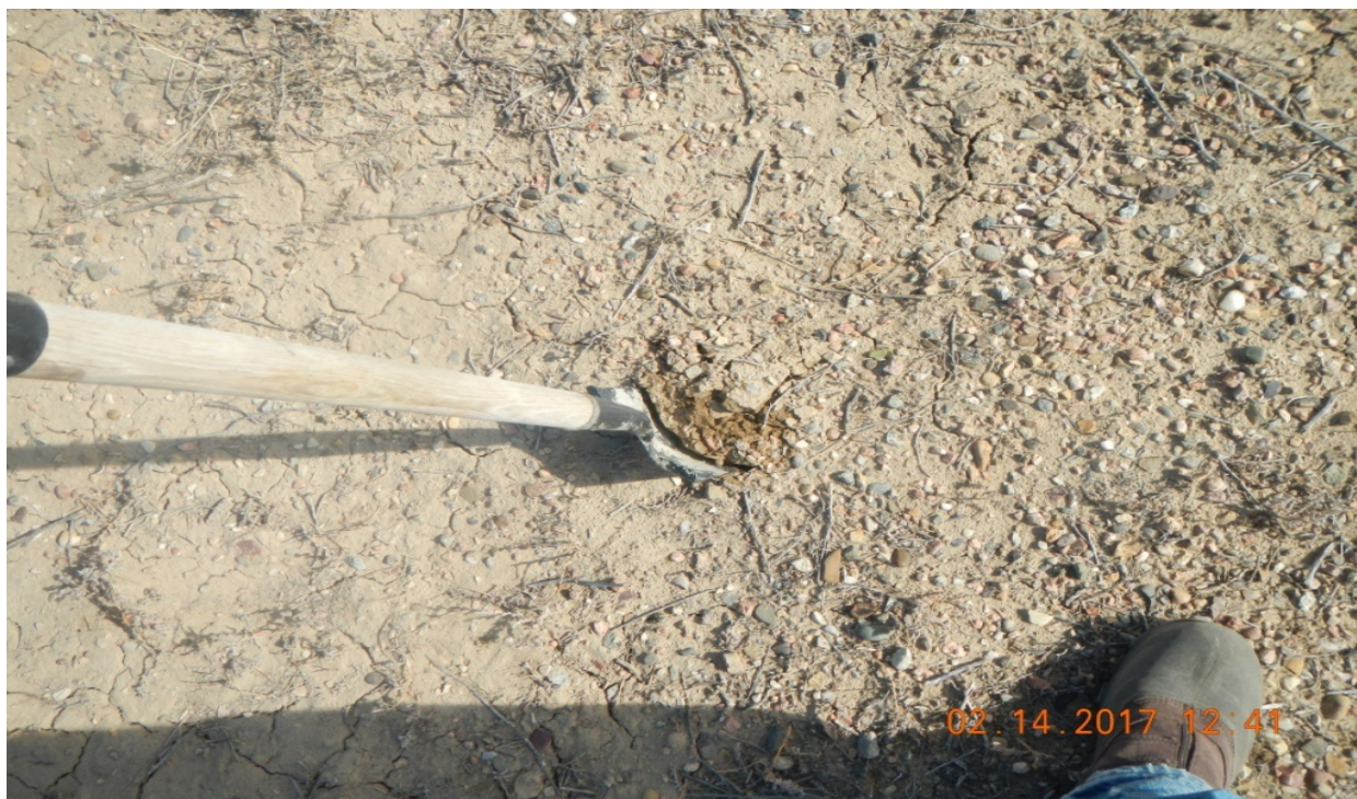
photo 3: The soils appeared to be compacted in the area where vegetation is not established.
