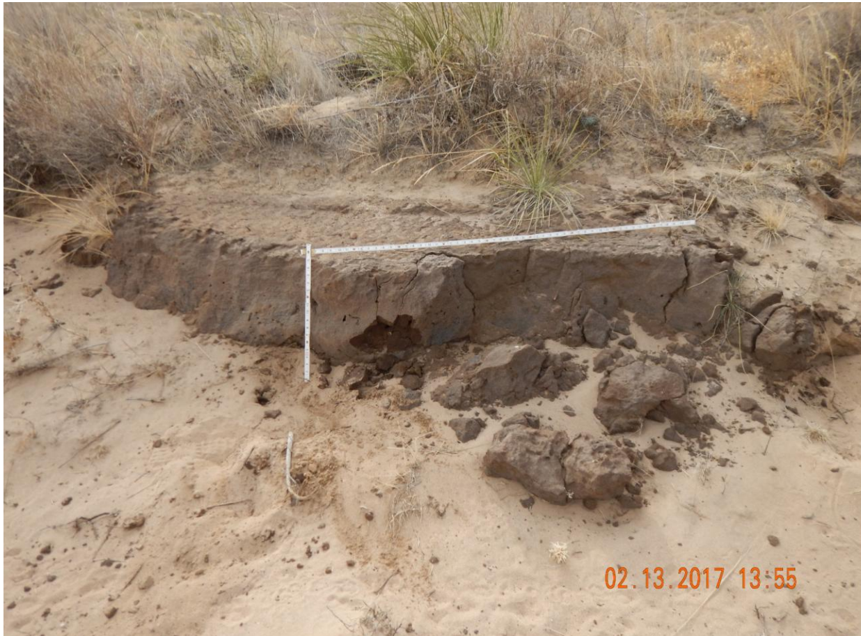
Photo 9: Photo taken from the east end of the location (refer to figures 7 and 8). Photo shows large portions of discolored and rigid soil. These soils need to be remediated or removed. 6' measuring stick for reference.
