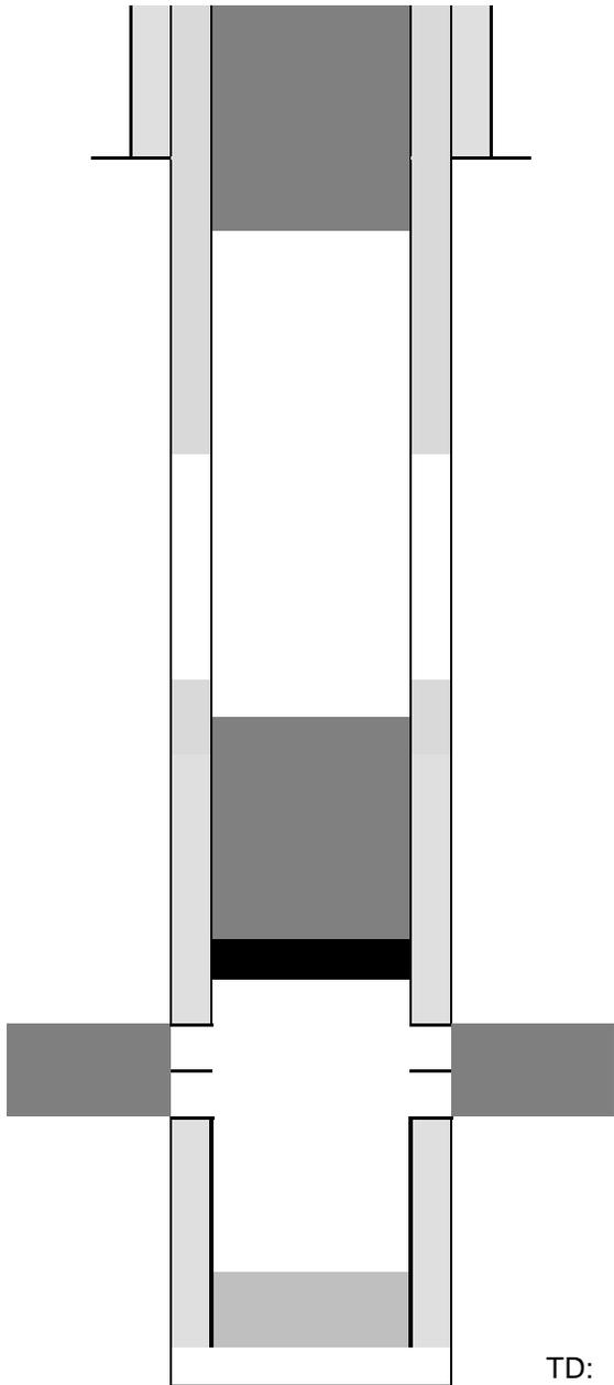
Cut surface casing off 6'-8' below surface.
