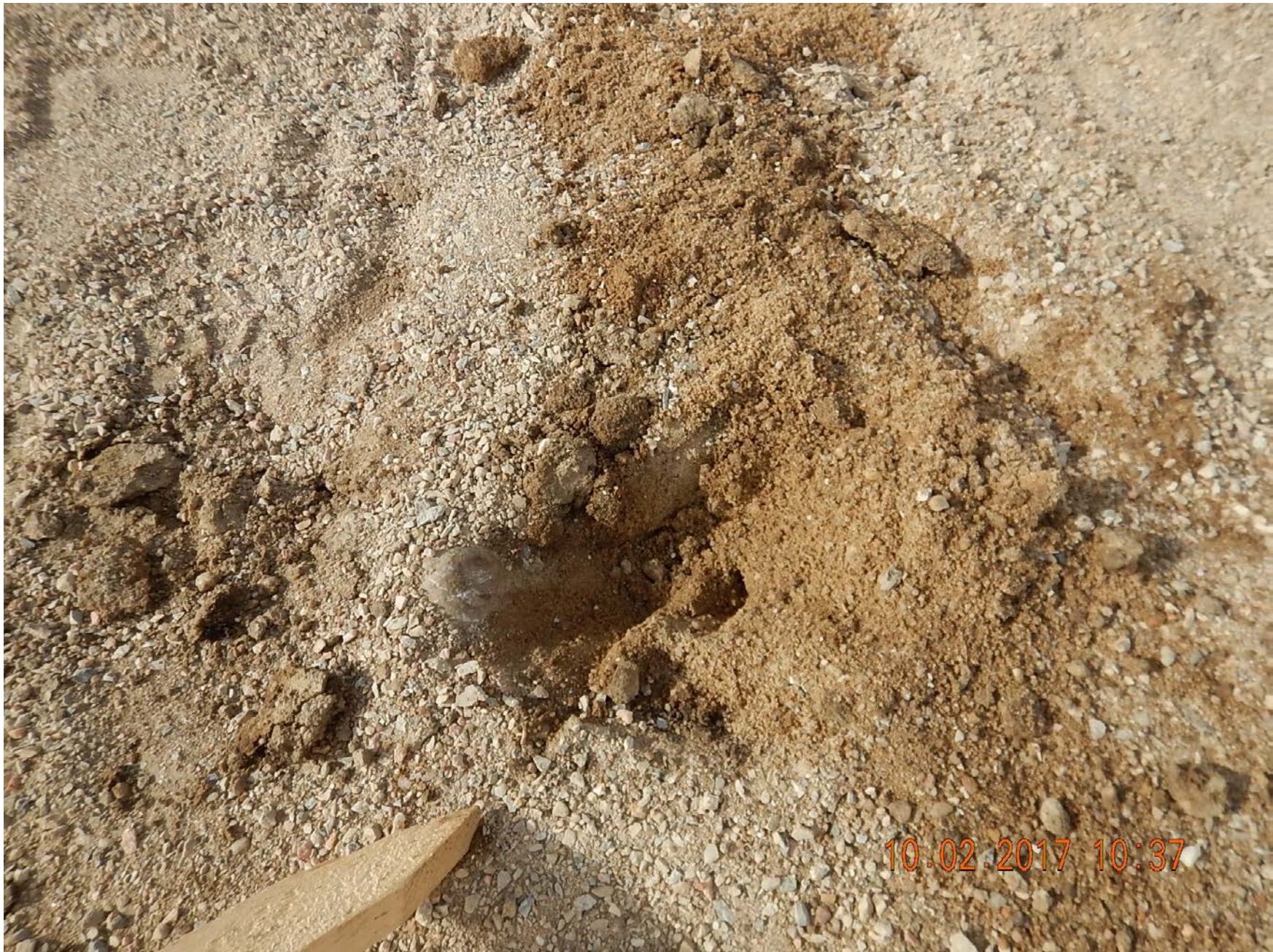
A small excavation in the secondary containment of heater treater. Base of secondary containment is composed of coarse to medium grained sand that appears to be highly permeable. A strong hydrocarbon odor was detected in this excavation.
