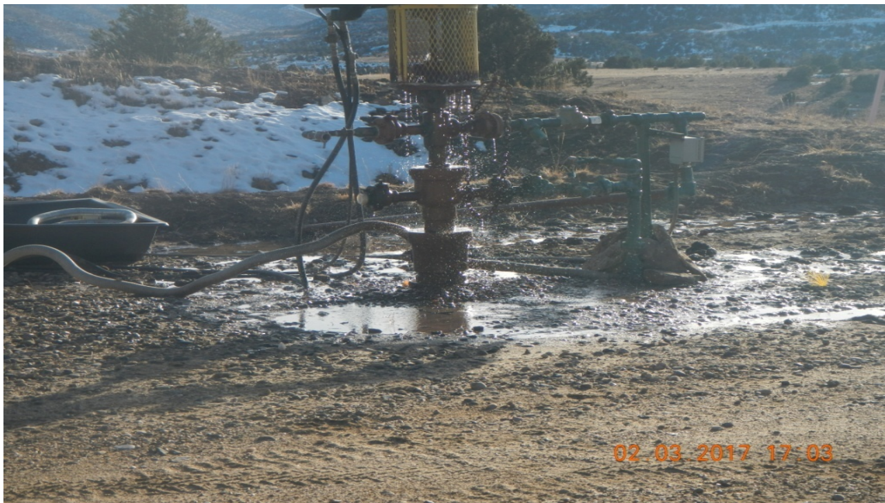
photo 4: Water was leaking from the wellhead.
