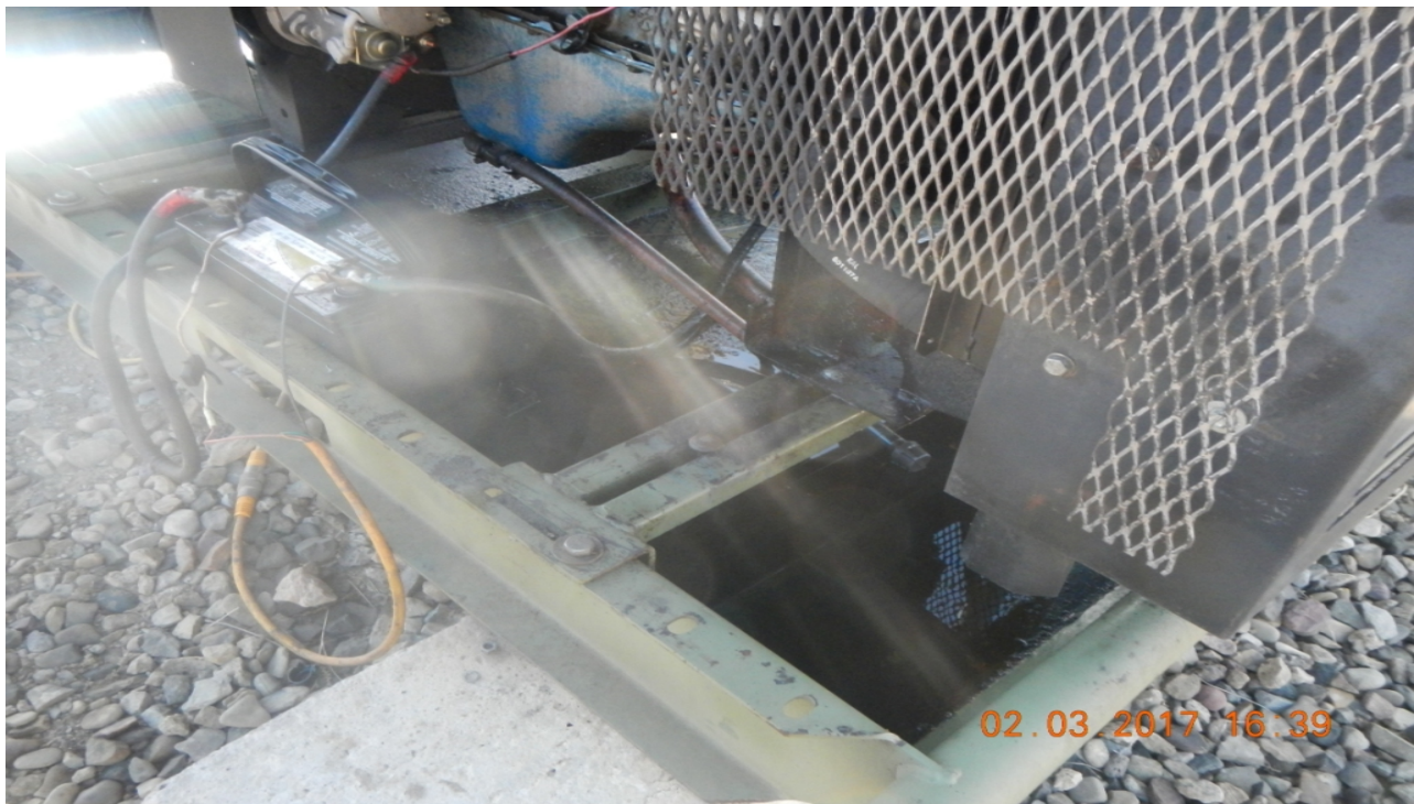
photo 4: There was oil noticed on the engine skid.
