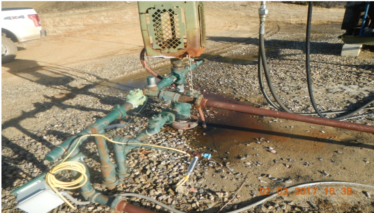
photo 3: There is a dripping water leak at the wellhead.
