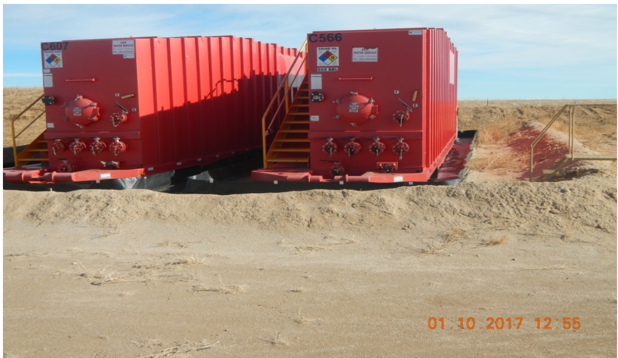
photo 6: Tanks are stored at the northeast side of the location. A berm is placed around the tanks.
