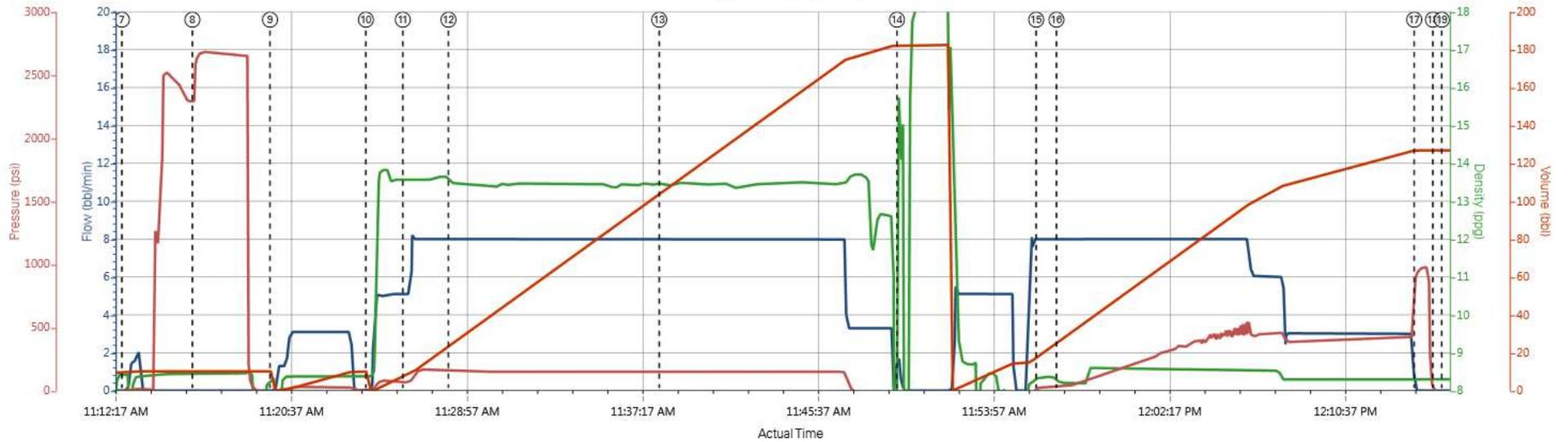
Comb Pump Rate (bbl/min) DH Density (ppg) PS Pump Press (psi) Pump Stg Tot (bbl)
