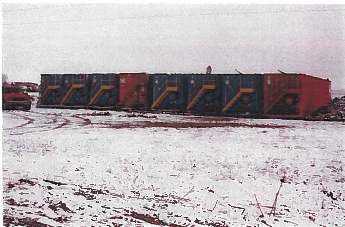
Photo 8 - A view of frac tanks mobilized to the site to store recovered liquids.
