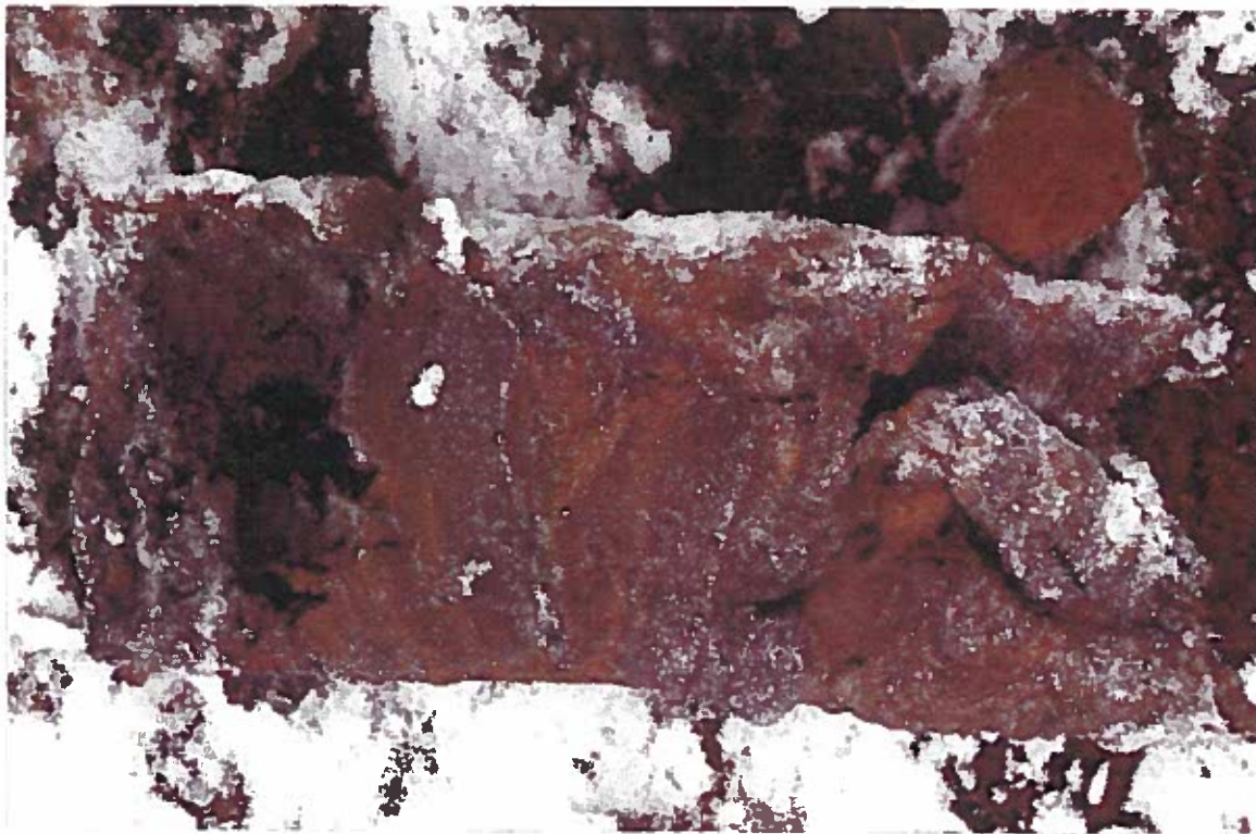
Photo 3 - View of section of removed drainage tile pipe. The pipe was clogged with clay.
