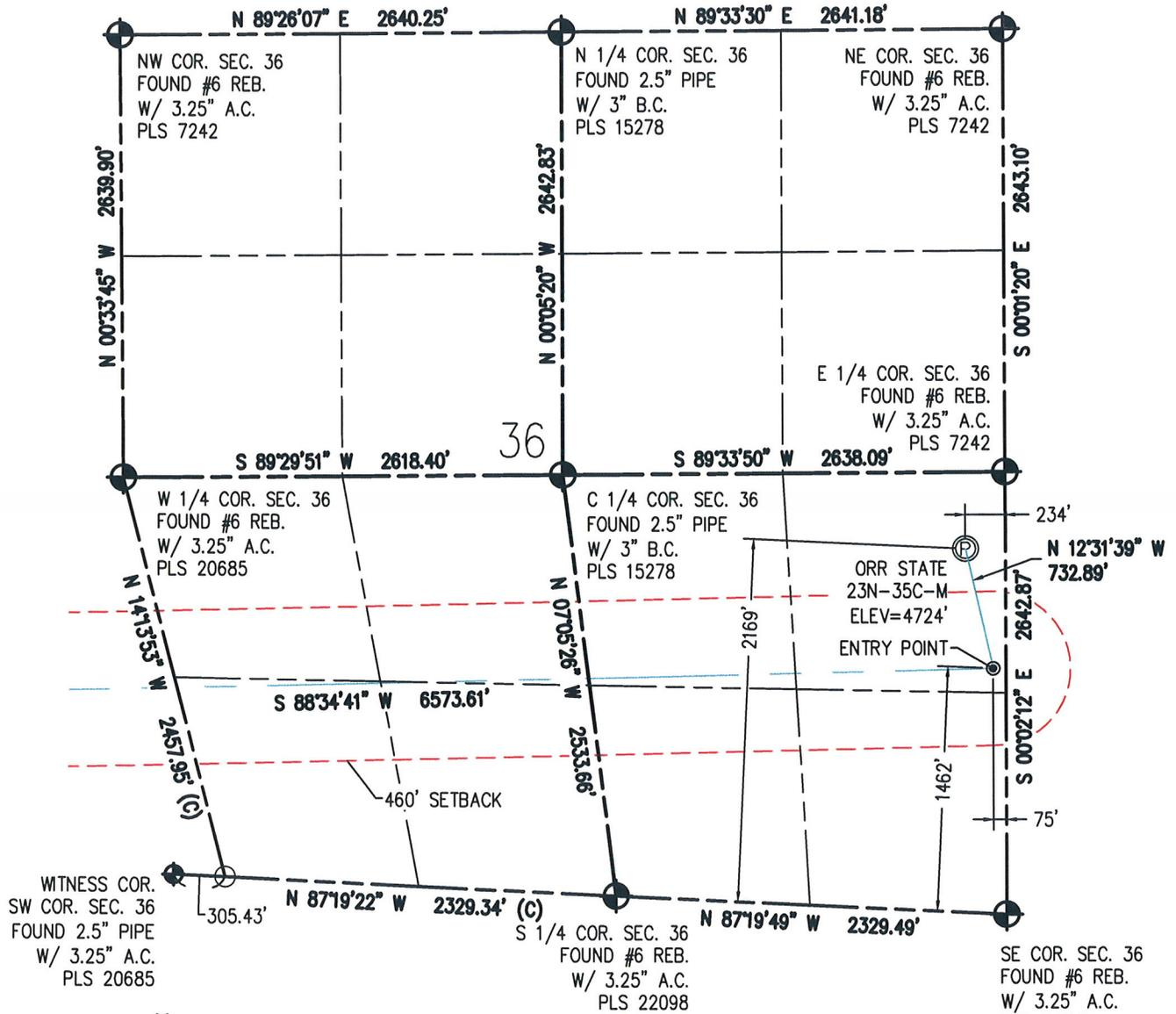
IN ACCORDANCE WITH A REQUEST FROM BRANDON LORENZ - SYNERGY RESOURCES, BASELINE ENGINEERING CORP. HAS DETERMINED THE LOCATION OF THE ORR STATE 23N-35C-M TO BE 2169' FSL AND 234' FEL, AS MEASURED AT NINETY (90) DEGREES FROM THE SECTION LINE OF SECTION 36, TOWNSHIP 6 NORTH, RANGE 67 WEST AND THE BOTTOM HOLE LOCATION TO BE 993' FSL AND 1665' FEL OF SECTION 35, TOWNSHIP 6 NORTH, RANGE 67 WEST, 6TH PRINCIPAL MERIDIAN, WELD COUNTY, COLORADO.
