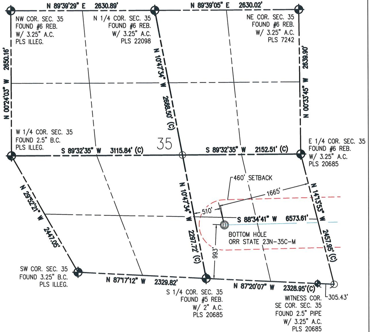
**N** IN ACCORDANCE WITH A REQUEST FROM BRANDON LORENZ - SYNERGY RESOURCES, BASELINE ENGINEERING CORP. HAS DETERMINED THE LOCATION OF THE ORR STATE 23N-35C-M TO BE 2169' FSL AND 234' FEL, AS MEASURED AT NINETY (90) DEGREES FROM THE SECTION LINE OF SECTION 36, TOWNSHIP 6 NORTH, RANGE 67 WEST AND THE BOTTOM HOLE LOCATION TO BE 993' FSL AND 1665' FEL OF SECTION 35, TOWNSHIP 6 NORTH, RANGE 67 WEST, 6TH PRINCIPAL MERIDIAN, WELD COUNTY, COLORADO.
