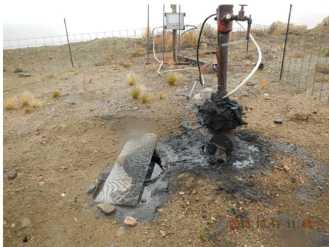
057-06080 Oil with sump and absorbent boom wrapped around well head.
