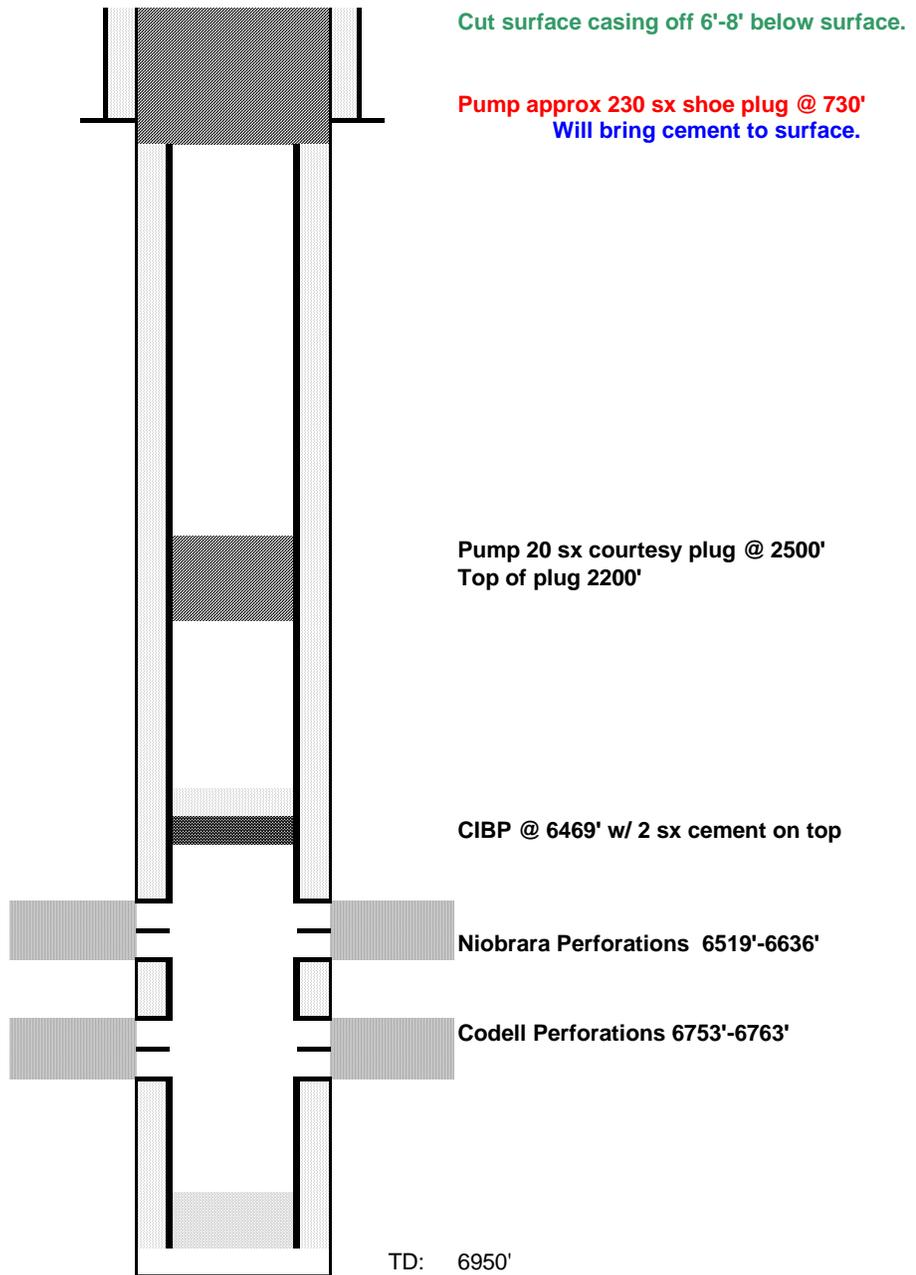
Cut surface casing off 6'-8' below surface.
