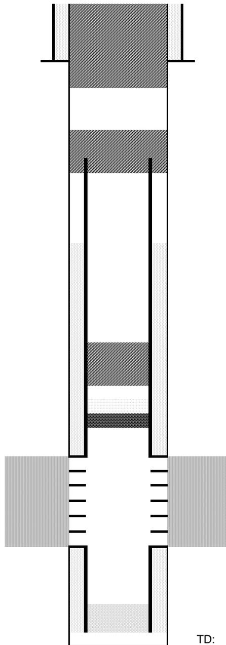
Cut surface casing off 6'-8' below surface.
