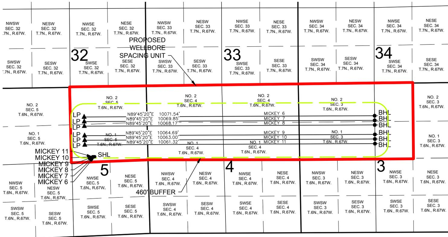
WELL MICKEY 6 TO BE LOCATED 2420' FNL AND 1843' FEL, SEC. 5, T6N, R67W
