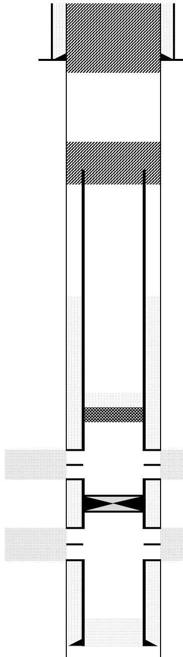
Cut surface casing off 6'-8' below surface.
