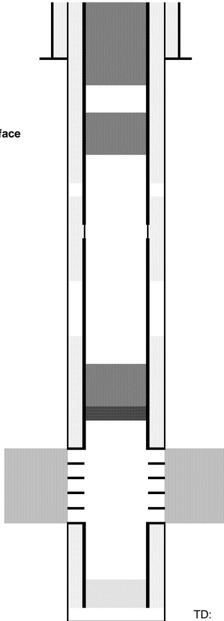
Cut surface casing off 6'-8' below surface.
