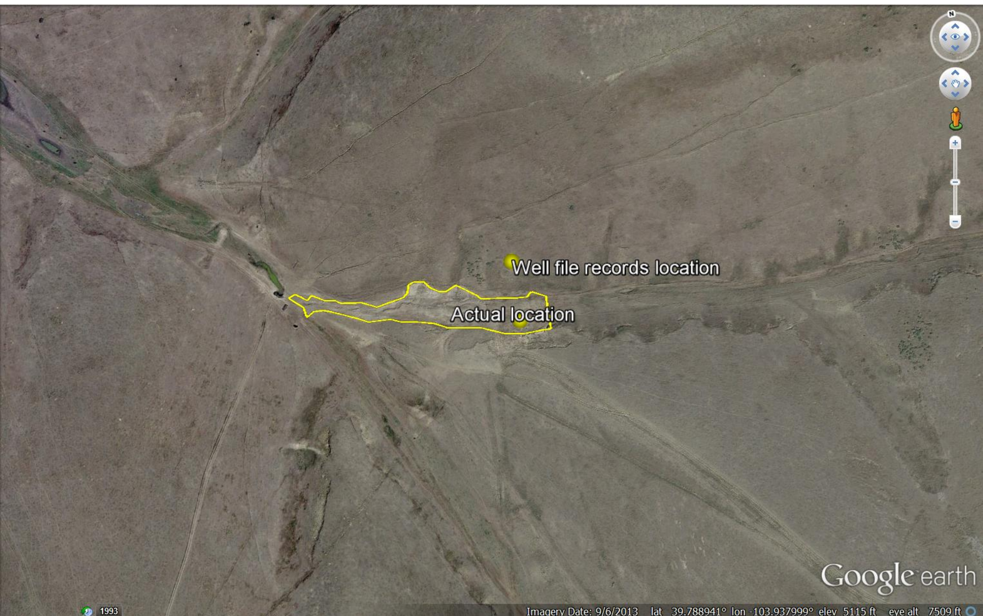
Figure 2: Most recent aerial imagery (2013) shows approximate outline of degradation within drainage. Approximate area of degradation is 1.3 acres.
