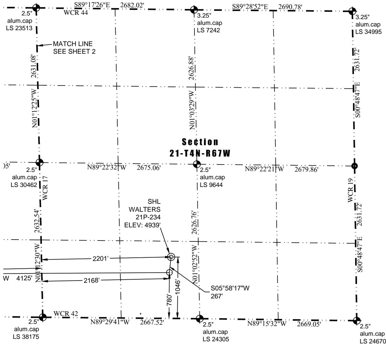
In accordance with a request from Mac Neumann of PDC Energy, Inc., Washburn Land Surveying, LLC has determined the location of the **WALTERS 21P-234** well site to be SHL: 1046' FSL and 2201' FWL, (BHL: 710' FSL and 1956' FEL), as measured at ninety (90) degrees from the section lines of Sections 21 and 20, Township 4 North, Range 67 West of the 6th Principal Meridian, Weld County Colorado.
