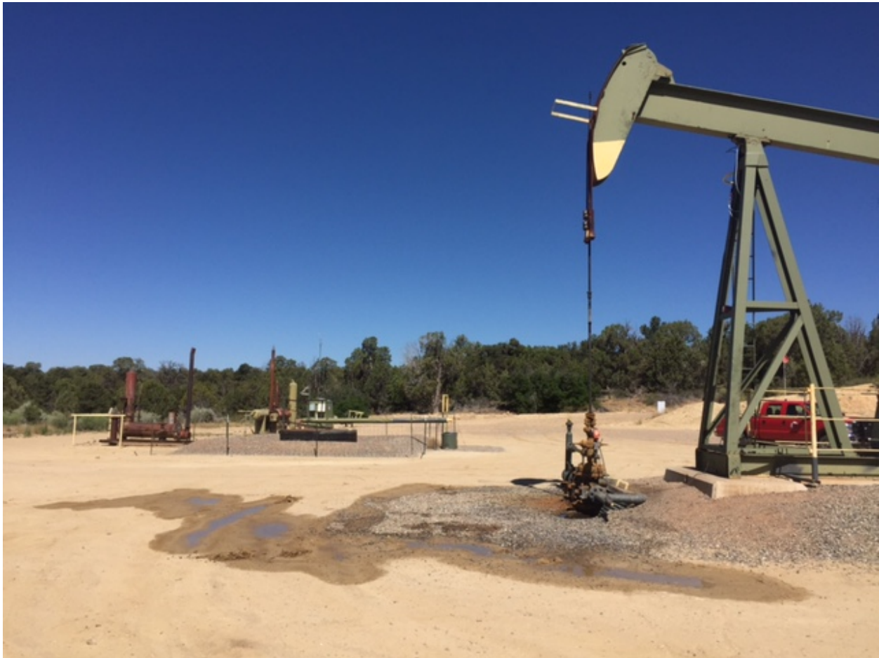
Figure 1. Fruitland Coal produced water spill area around the wellhead. Spill resulted from a wellhead packing leak.
