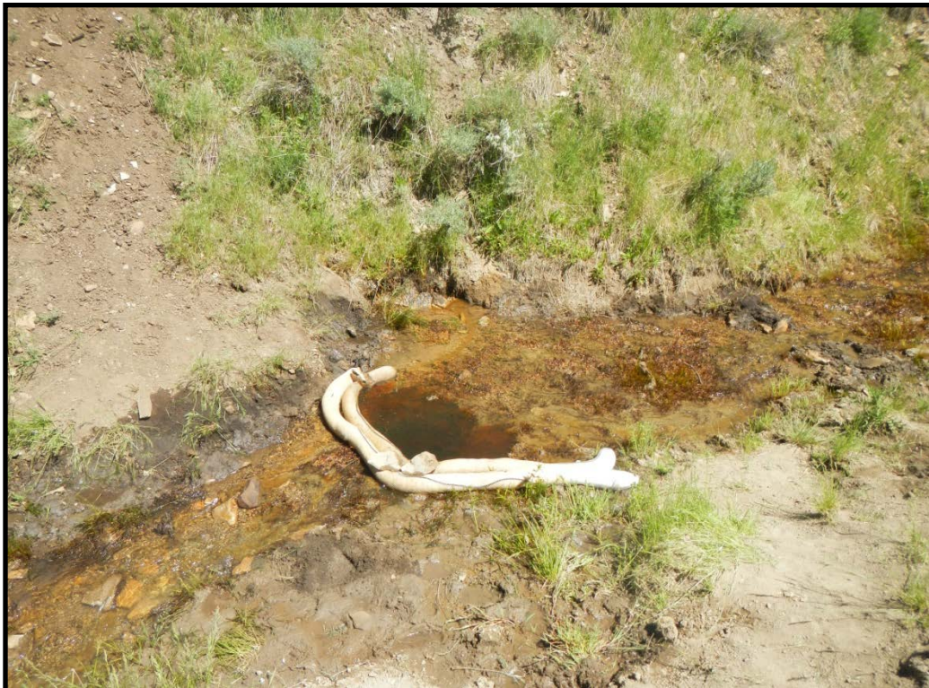
Close-up showing one of the Springs and free-product retained by booms. Natural drainage is dry upgradient of Springs. Continuous flow downgradient. Approximately one mile to stock pond.
