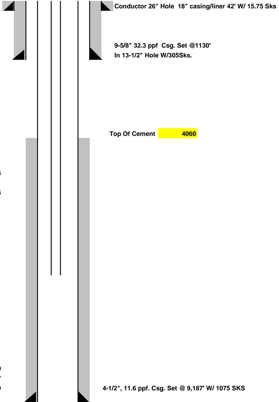
Conductor 26" Hole 18" casing/liner 42' W/ 15.75 Sks
