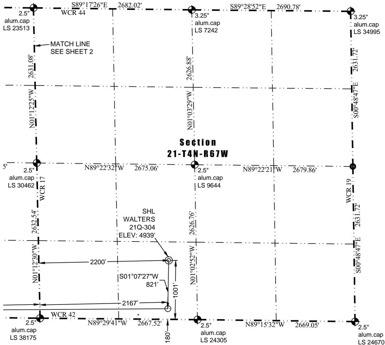
In accordance with a request from Mac Neumann of PDC Energy, Inc., Washburn Land Surveying, LLC has determined the location of the **WALTERS 21Q-304** well site to be SHL: 1001' FSL and 2200' FWL, (BHL: 110' FSL and 1961' FEL), as measured at ninety (90) degrees from the section lines of Sections 21 and 20, Township 4 North, Range 67 West of the 6th Principal Meridian, Weld County Colorado.
