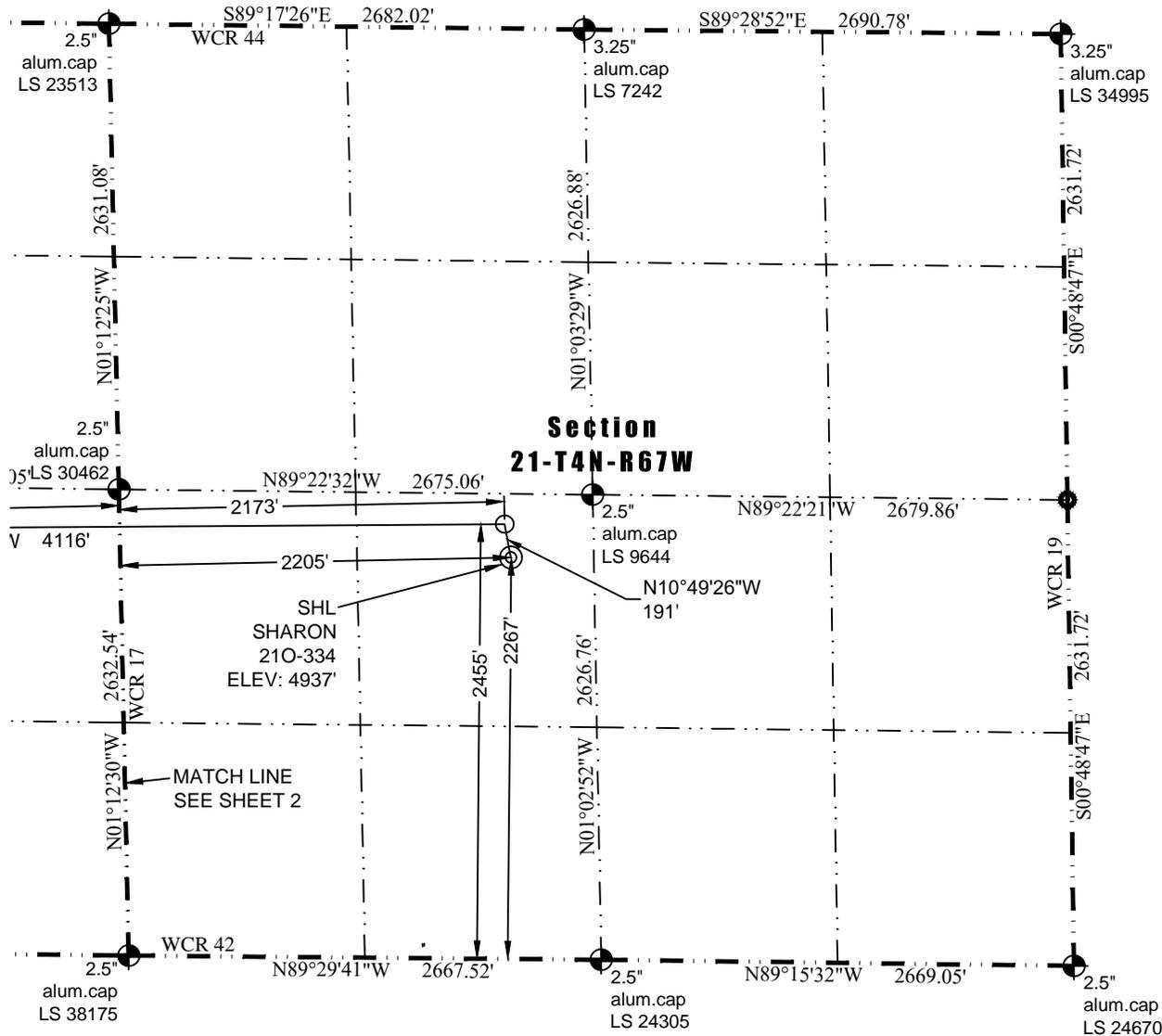
In accordance with a request from Mac Neumann of PDC Energy, Inc., Washburn Land Surveying, LLC has determined the location of the **SHARON 210-334** well site to be SHL: 2267' FSL and 2205' FWL, (BHL: 2385' FSL and 1943' FEL), as measured at ninety (90) degrees from the section lines of Sections 21 and 20, Township 4 North, Range 67 West of the 6th Principal Meridian, Weld County Colorado.
